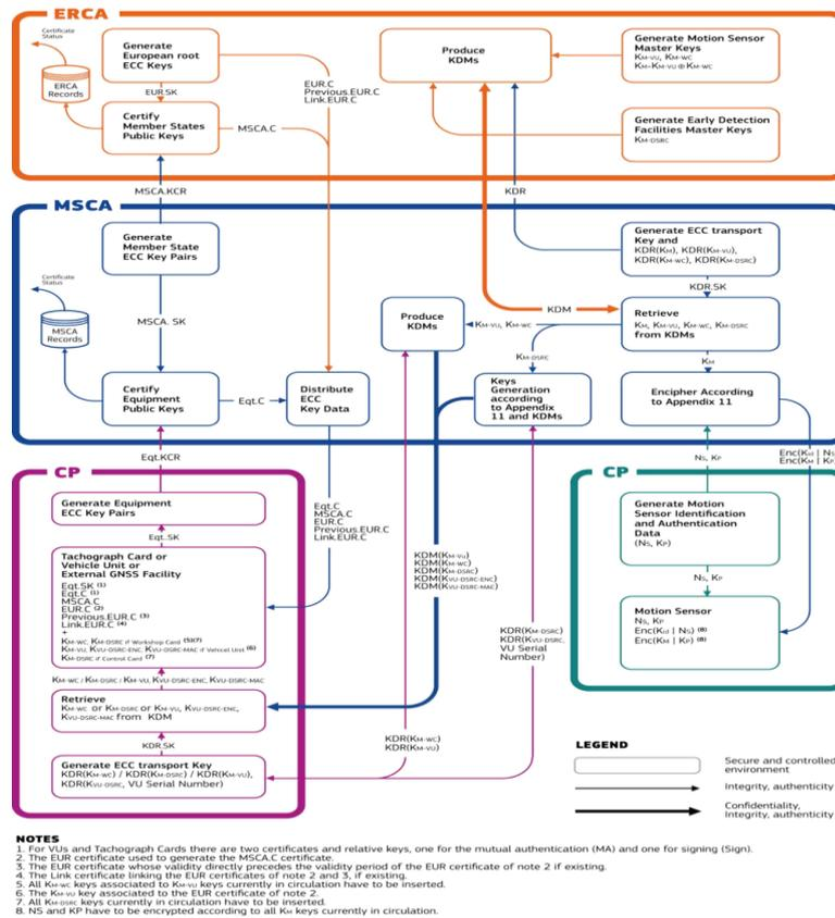
Figure 1 Smart Tachograph PKI and Symmetric Key Infrastructure
