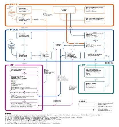
Figure 1 Smart Tachograph PKI and Symmetric Key Infrastructure
